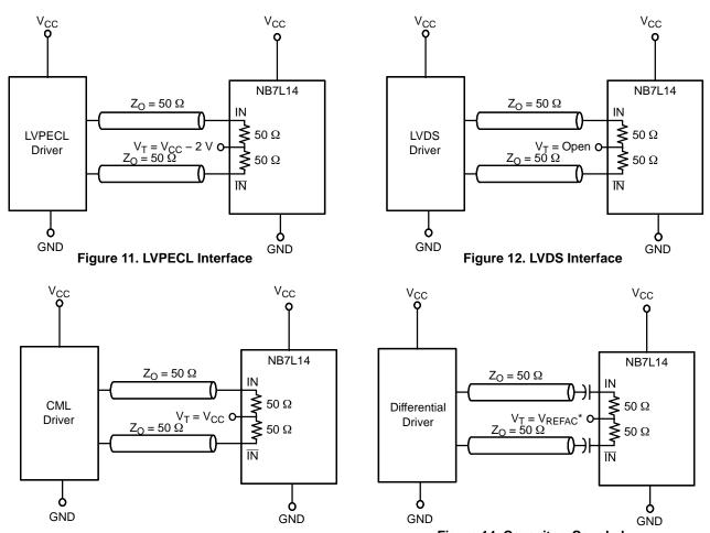
Figure 13. Standard 50  $\Omega$  Load CML Interface
