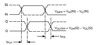
Figure 10. AC Reference Measurement
