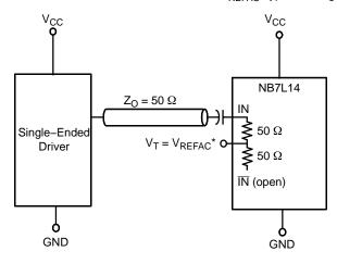
Figure 15. Capacitor–Coupled Differential Interface (V<sub>T</sub> Connected to External V<sub>REFAC</sub>)
