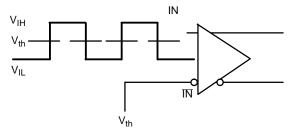
Figure 5. Differential Input Driven Single-Ended
