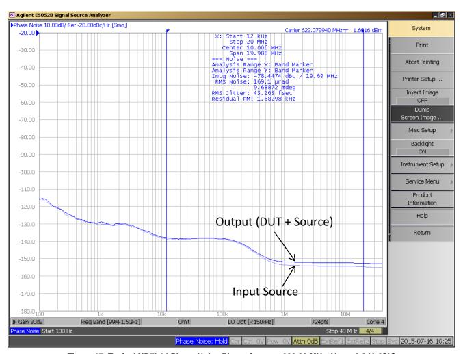
Figure 17. Typical NB7L14 Phase Noise Plot at f<sub>Carrier</sub> = 622.08 MHz, V<sub>CC</sub> = 3.3 V, 25°C
