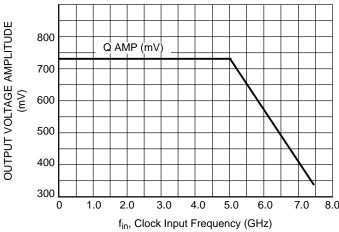
Figure 3. CLOCK Output Voltage Amplitude (V<sub>OUTPP</sub>) vs. Input Frequency (f<sub>in</sub>) at Ambient Temperature (Typ)
