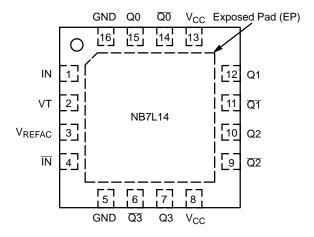
Figure 2. QFN-16 Pinout (Top View)
