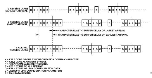
Figure 56. Lane Alignment During ILAS
