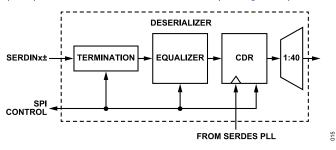
Figure 49. Deserializer Block Diagram
