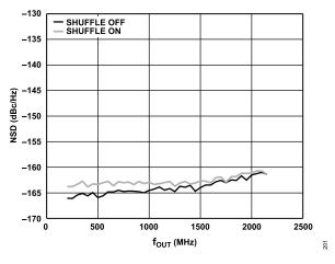
Figure 25. Single-Tone NSD Measured at 70 MHz vs. f<sub>OUT</sub>, 11796.48 MHz f<sub>DAC</sub>, 16-Bit Resolution, Shuffle Off vs. Shuffle On
