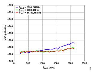
Figure 26. Single-Tone NSD Measured at 70 MHz vs. f<sub>OUT</sub> over f<sub>DAC</sub>, 16-Bit Resolution, Shuffle On
