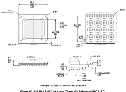
Figure 90. 144-Ball Ball Grid Array, Thermally Enhanced [BGA\_ED] (BP-144-1) Dimensions shown in millimeters
