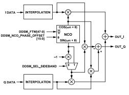
Figure 76. NCO Modulator Block Diagram
