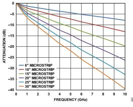
Figure 54. Insertion Loss of 50 Ω Microstrips on FR4
