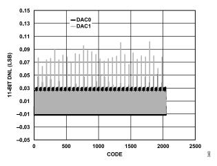
Figure 41. DNL, I<sub>OUTFS</sub> = 20 mA, 11-Bit Resolution
