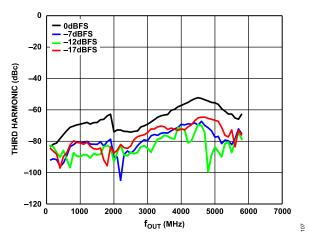
Figure 7. Third Harmonic (dBc) vs. f<sub>OUT</sub> over Digital Scale (Mode 1),12 GHz DAC Sample Rate, Channel Interpolation 4×, Main Interpolation 8×
