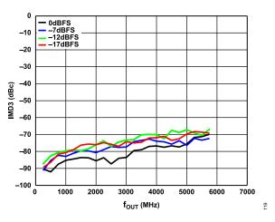
Figure 19. IMD3 vs. f<sub>OUT</sub> over Digital Scale (Mode 1), 12 GHz DAC Sample Rate, Channel Interpolation 4×, Main Interpolation 8×, 1 MHz Tone Spacing
