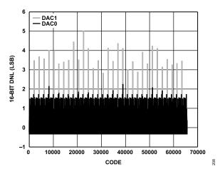
Figure 33. DNL, I<sub>OUTFS</sub> = 26 mA, 16-Bit Resolution
