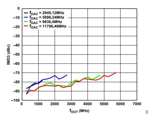
Figure 22. IMD3 vs. f<sub>OUT</sub> over f<sub>DAC</sub> (Mode 2), Channel Interpolation 4×, Main Interpolation 8×, 1 MHz Tone Spacing
