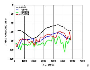
Figure 16. Third Harmonic (dBc) vs. f<sub>OUT</sub> over Digital Scale (Mode 9),12 GHz DAC Sample Rate, Channel Interpolation 1×, Main Interpolation 12×
