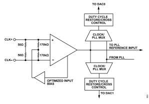
Figure 86. Clock Receiver Input Simplified Equivalent Circuit
