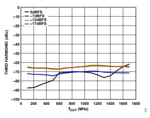
Figure 13. Third Harmonic (dBc) vs. f<sub>OUT</sub> over Digital Scale (Mode 17), 3.4 GHz DAC Sample Rate, Channel Interpolation 1×, Main Interpolation 1×, 11-Bit Resolution
