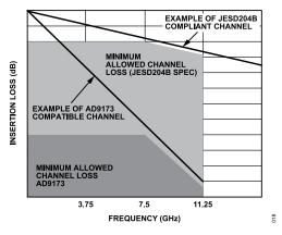
Figure 52. Insertion Loss Allowed
