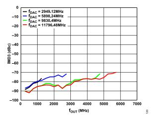
Figure 20. IMD3 vs. f<sub>OUT</sub> over f<sub>DAC</sub> (Mode 1), Channel Interpolation 4×, Main Interpolation 8×, 1 MHz Tone Spacing, -7 dB Digital Scale
