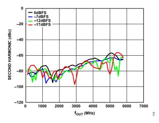
Figure 15. Second Harmonic (dBc) vs. f<sub>OUT</sub> over Digital Scale (Mode 9),12 GHz DAC Sample Rate, Channel Interpolation 1×, Main Interpolation 12×
