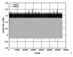
Figure 37. DNL, I<sub>OUTFS</sub> = 15.6 mA, 16-Bit Resolution
