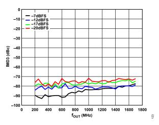
Figure 23. IMD3 vs. f<sub>OUT</sub> over Digital Scale (Mode 17), 3.4 GHz DAC Sample Rate, Channel Interpolation 1×, Main Interpolation 1×, 1 MHz Tone Spacing, 11-Bit Resolution
