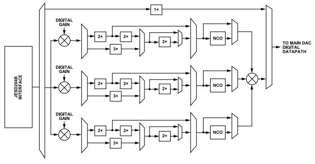
Figure 69. Block Diagram of the Channel Digital Datapath per the Main DAC Output
