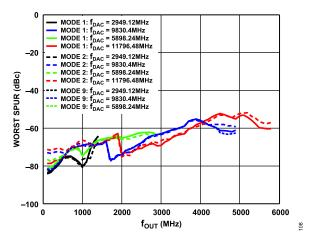
Figure 8. Worst Spur (dBc) vs. four over fDAC (All Modes), 0 dB Digital Scale
