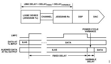
Figure 59. JESD204B Link Delay = Fixed Delay + Variable Delay
