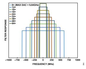
Figure 67. Band Responses of Total Interpolation Rates for 8×, 12×, 16×, 18×, 24×, 32×, 36×, 48×, and 64× at a 12 GHz DAC Rate, 16-Bit Resolution (Unless Otherwise Noted)
