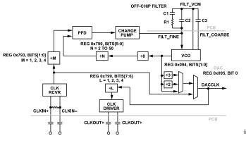
Figure 88. DAC PLL and Clock Path Block Diagram
