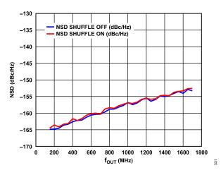
Figure 31. Single-Tone NSD Measured at 70 MHz vs. f<sub>OUT</sub>, 3.4 GHz f<sub>DAC</sub>, 11-Bit Resolution, Shuffle Off vs. Shuffle On
