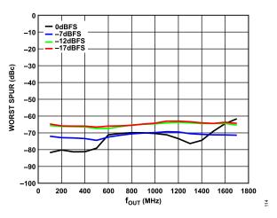
Figure 14. Worst Spur (dBc) vs. f<sub>OUT</sub> over Digital Scale (Mode 17),3.4 GHz DAC Sample Rate, Channel Interpolation 1×, Main Interpolation 1×, 11-Bit Resolution
