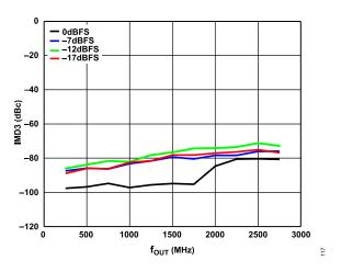
Figure 17. IMD3 vs. f<sub>OUT</sub> over Digital Scale (Mode 0) 6 GHz DAC Sample Rate, Channel Interpolation 2×, Main Interpolation 8×, 1 MHz Tone Spacing
