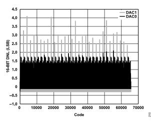
Figure 35. DNL, I<sub>OUTFS</sub> = 20 mA, 16-Bit Resolution
