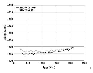
Figure 28. Single-Tone NSD Measured at 70 MHz vs. f<sub>OUT</sub>, 11796.48 MHz f<sub>DAC</sub>, 12-Bit Resolution, Shuffle Off vs. Shuffle On
