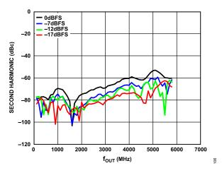
Figure 6. Second Harmonic (dBc) vs. f<sub>OUT</sub> over Digital Scale (Mode 1),12 GHz DAC Sample Rate, Channel Interpolation 4×, Main Interpolation 8×
