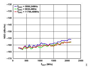
Figure 30. Single-Tone NSD Measured at 10% Offset from  $f_{OUT}$  vs.  $f_{OUT}$  over  $f_{DAC}$ , 12-Bit Resolution, Shuffle On
