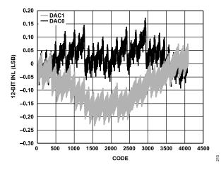
Figure 40. INL, I<sub>OUTFS</sub> = 20 mA, 12-Bit Resolution
