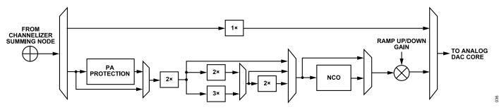
Figure 72. Block Diagram of the Main Digital Datapath per Main DAC Output
