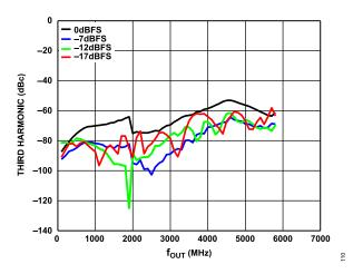
Figure 10. Third Harmonic (dBc) vs. f<sub>OUT</sub> over Digital Scale (Mode 2),12 GHz DAC Sample Rate, Channel Interpolation 4×, Main Interpolation 8×
