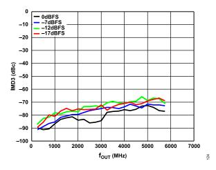
Figure 24. IMD3 vs. f<sub>OUT</sub> over Digital Scale (Mode 9), 12 GHz DAC Sample Rate, Channel Interpolation 1×, Main Interpolation 12×, 1 MHz Tone Spacing
