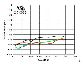
Figure 5. Worst Spur (dBc) vs. f<sub>OUT</sub> over Digital Scale (Mode 0), 6 GHz DAC Sample Rate, Channel Interpolation 2×, Main Interpolation 8×
