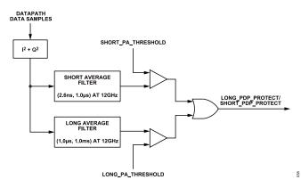
Figure 74. PDP Block Diagram
