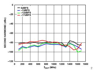
Figure 12. Second Harmonic (dBc) vs. f<sub>OUT</sub> over Digital Scale (Mode 17),3.4 GHz DAC Sample Rate, Channel Interpolation 1×, Main Interpolation 1×, 11-Bit Resolution
