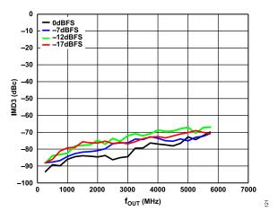
Figure 21. IMD3 vs. f<sub>OUT</sub> over Digital Scale (Mode 2), 12 GHz DAC Sample Rate, Channel Interpolation 4×, Main Interpolation 8×, 1 MHz Tone Spacing
