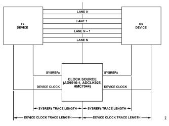
Figure 85. SYSREF± Signal and Device Clock Trace Length
