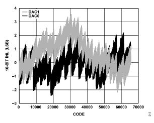
Figure 38. INL, I<sub>OUTFS</sub> = 15.6 mA, 16-Bit Resolution
