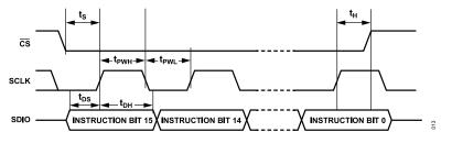
Figure 47. Timing Diagram for Serial Port Register Write
