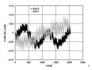
Figure 42. INL, I<sub>OUTFS</sub> = 20 mA, 11-Bit Resolution
