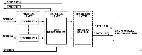
Figure 48. Functional Block Diagram of Serial Link Receiver
