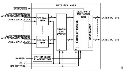
Figure 55. Data Link Layer Block Diagram
