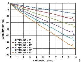
Figure 53. Insertion Loss of 50  $\Omega$  Striplines on FR4
