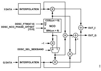
Figure 71. NCO Modulator Block Diagram
