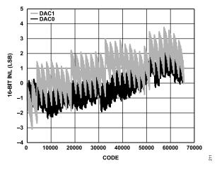
Figure 36. INL, I<sub>OUTFS</sub> = 20 mA, 16-Bit Resolution
