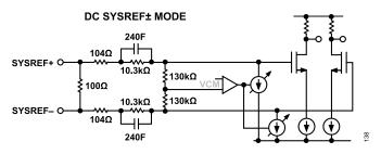
Figure 57. DC-Coupled SYSREF± Receiver Circuitry
