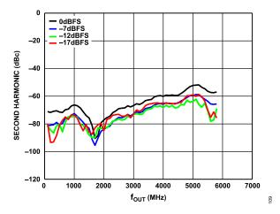
Figure 9. Second Harmonic (dBc) vs. f<sub>OUT</sub> over Digital Scale (Mode 2),12 GHz DAC Sample Rate, Channel Interpolation 4×, Main Interpolation 8×
