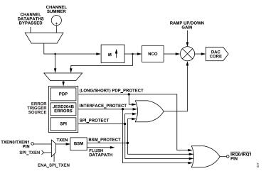
Figure 73. Block Diagram of Downstream Protection Triggers
