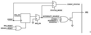
Figure 81. Simplified Schematic of IRQx Circuitry
