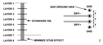
Figure 82. Minimizing Stub Effect and Adding Ground Vias for Differential Stripline Traces
