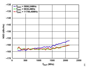
Figure 29. Single-Tone NSD Measured at 70 MHz vs. f<sub>OUT</sub> over f<sub>DAC</sub>, 12-Bit Resolution, Shuffle On
