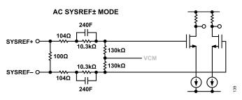
Figure 58. AC-Coupled SYSREF± Receiver Circuitry
