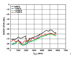
Figure 11. Worst Spur(dBc) vs. f<sub>OUT</sub> over Digital Scale (Mode 2),12 GHz DAC Sample Rate, Channel Interpolation 4×, Main Interpolation 8×
