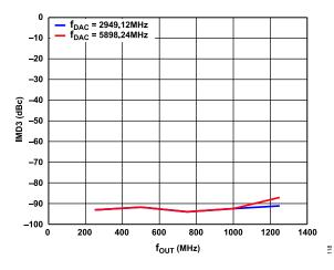
Figure 18. IMD3 vs. f<sub>OUT</sub> over f<sub>DAC</sub> (Mode 0), Channel Interpolation 2×, Main Interpolation 8×, 1 MHz Tone Spacing
