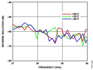
Figure 28. Reverse Isolation vs. Frequency for Various Temperatures
