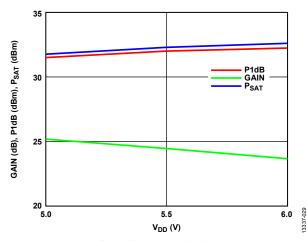
Figure 29. Gain, P1dB, and PSAT vs. Supply Voltage (VDD) at 38.5 GHz
