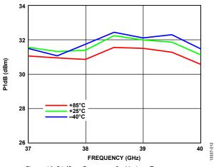
Figure 12. P1dB vs. Frequency for Various Temperatures
