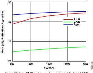
Figure 30. Gain, P1dB, and PSAT vs. Supply Current (IDD) at 38.5 GHz
