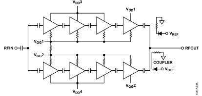
Figure 33. GaAs, pHEMT, 1 W MMIC Power Amplifier Block Diagram
