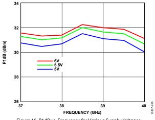
Figure 15. P1dB vs. Frequency for Various Supply Voltages
