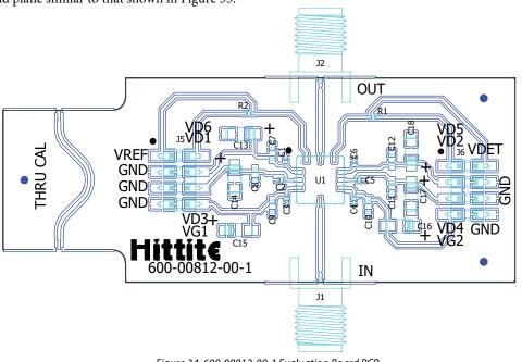
Figure 34. 600-00812-00-1 Evaluation Board PCB
