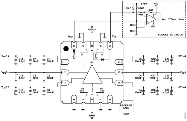
Figure 35. Typical Application Circuit
