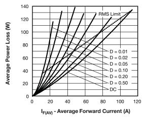
Fig. 6 - Forward Power Loss Characteristics
