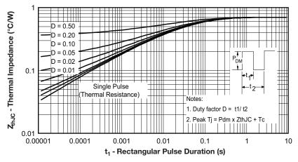
Fig. 4 - Maximum Thermal Impedance Z<sub>thJC</sub> Characteristics
