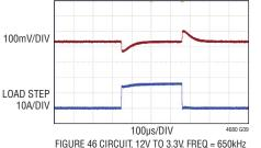
FIGURE 46 CIRCUIT, 12V TO 3.3V, FREQ = 650kHz  $C_{OUT} = 470\mu F \times 2 \text{ POSCAP}$ , 100 $\mu F \times 4 \text{ CERAMIC}$   $R_{COMP} = 20k$ , EA-Gm = 3.02ms, COMPna = 3.3nF, COMPnb = 68pF $I_{LIM}$  LOW,  $V_{OUT}$  RANGE HIGH
