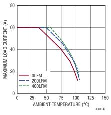
Figure 43. 12V to 1.8V Derating Curve, No Heat Sink
