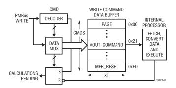
Figure 32. Write Command Data Processing
