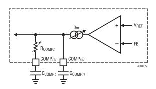
Figure 27. Programmable Loop Compensation
