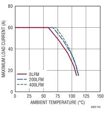
Figure 40. 12V to 0.9V Derating Curve, No Heat Sink
