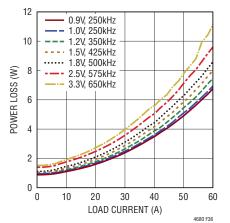
Figure 36. 8V<sub>IN</sub> Power Loss Curve
