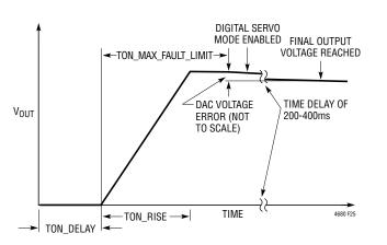
Figure 25. Timing Controlled V<sub>OUT</sub> Rise
