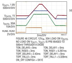
Single Channel Load Transient Response 50% (15A) to 100% (30A) Load Step, 15A/ $\mu$ s V<sub>IN</sub> = 12V, V<sub>OUT</sub> = 1.2V, f<sub>SW</sub> = 350kHz
