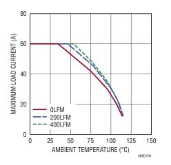
Figure 41. 5V to 1.8V Derating Curve, No Heat Sink
