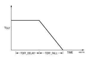
Figure 26. TOFF\_DELAY and TOFF\_FALL
