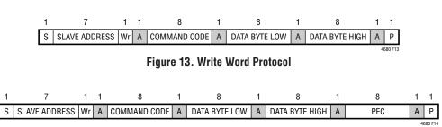
Figure 14. Write Word Protocol with PEC
