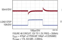
$\begin{aligned} & \text{COMP} = 17\text{k}, \text{EA-GM} = 3.69\text{ms}, \\ & \text{COMP}\text{a} = 3.3\text{nF}, \text{COMP}\text{a} = 68\text{pF} \\ & \text{I_{LIM}} \text{ LOW}, \text{V}_{\text{OUT}} \text{ RANGE LOW} \end{aligned}$
