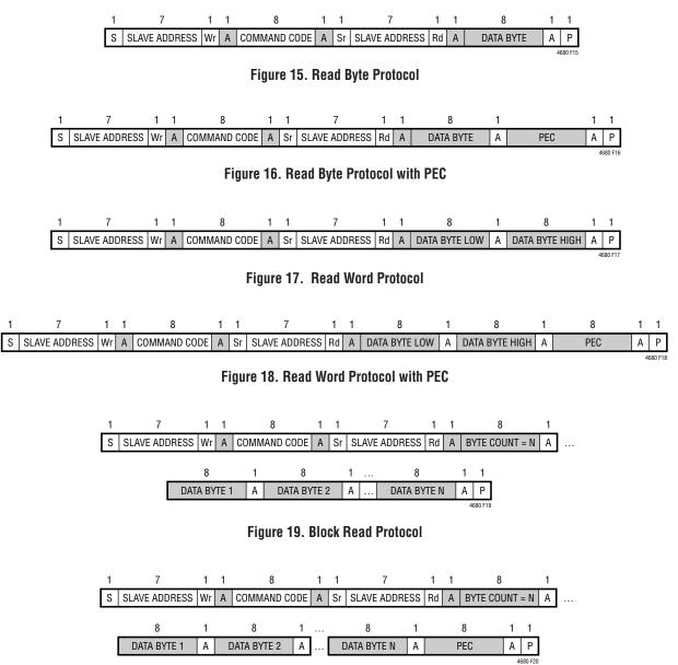
Figure 20. Block Read Protocol with PEC
