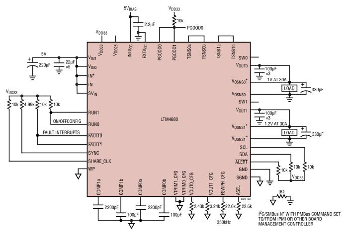
Figure 48. 1V and 1.2V Outputs Generated from 5V Power Input and Providing I<sup>2</sup>C/SMBus/PMBus Serial Interface
