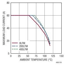
Figure 38. 5V to 0.9V Derating Curve, No Heat Sink
