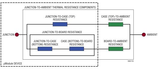
Figure 34. Graphical Representation of JESD51-12 Thermal Coefficients
