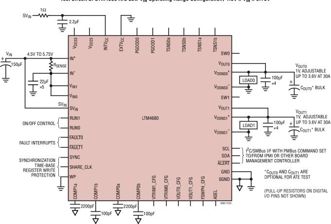
Test Circuit 2. LTM4680 ATE Low V<sub>IN</sub> Operating Range Configuration,  $4.5V \le V_{IN} \le 5.75V$
