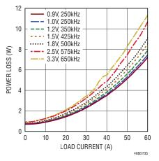
Figure 35. 5V<sub>IN</sub> Power Loss Curve
