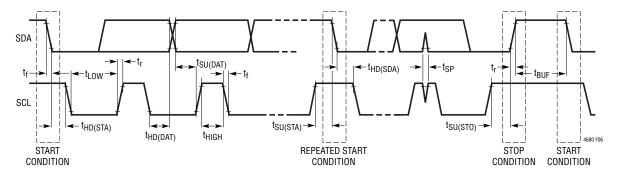
Figure 6. PMBus Timing Diagram
