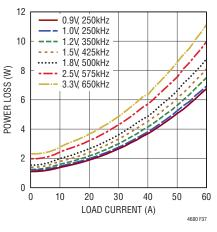
Figure 37. 12V<sub>IN</sub> Power Loss Curve
