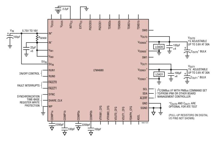
Test Circuit 1. LTM4680 ATE High  $V_{IN}$  Operating Range Configuration, 5.75V  $\leq V_{IN} \leq 16V$
