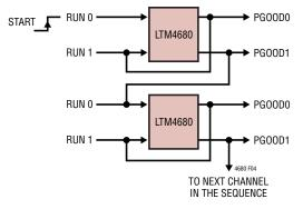
Figure 4. Event (Voltage) Based Sequencing
