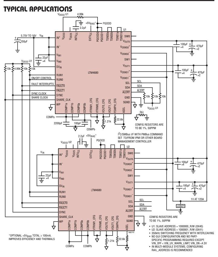
Figure 47. Two Paralleled LTM4680 Producing 1V<sub>OUT</sub> at 120A. Integrated Power System Management Features Accessible Over 2-Wire I<sup>2</sup>C/SMBus/PMBus Serial Interface
