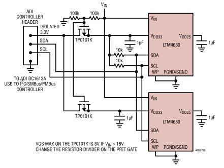
Figure 30. Controller Connection
