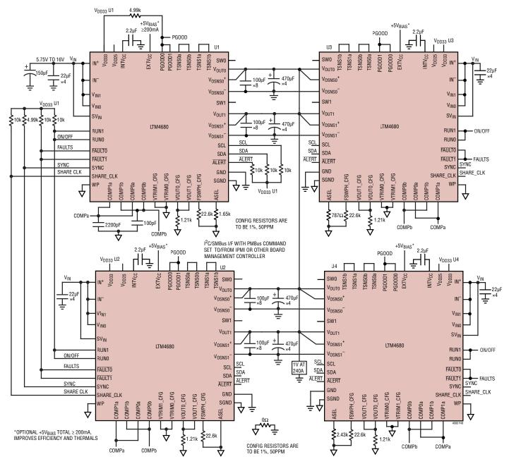
Figure 49. 8-Phase Operation with Four LTM4680 Producing 1V at 240A. Power System Management Features Accessible Through LTM4680 Over 2-Wire I<sup>2</sup>C/SMBus/PMBus Serial Interface
