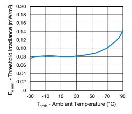
Fig. 9 - Sensitivity vs. Ambient Temperature
