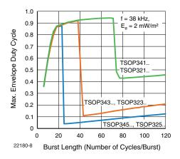
Fig. 8 - Maximum Envelope Duty Cycle vs. Burst Length
