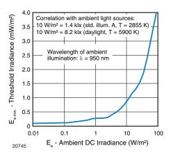
Fig. 6 - Sensitivity in Bright Ambient
