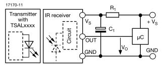
$R_{\rm 1}$  and  $C_{\rm 1}$  recommended to reduce supply ripple for  $V_{\rm S}$  < 2.8~V
