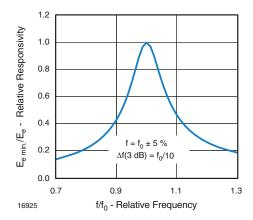
Fig. 5 - Frequency Dependence of Responsivity
