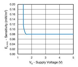
Fig. 12 - Sensitivity vs. Supply Voltage
