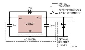
Figure 1c. A Schottky Diode Can Limit the Transient Caused by a Fast Rising  $V_{\text{IN}}$  to Safe Levels
