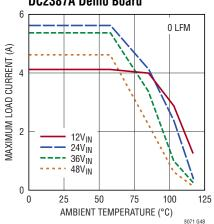
Derating, V<sub>OUT</sub> = -8V, BIAS Tied to LTM8071 GND DC2387A Demo Board
