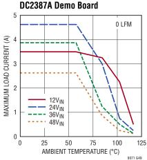
Derating, V<sub>OUT</sub> = -12V, BIAS Tied to LTM8071 GND DC2387A Demo Board
