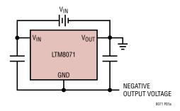
Figure 1a. The LTM8071 Can Be Used to Generate a Negative Voltage
