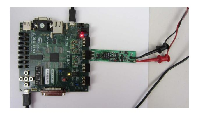
Figure 1. Campbell Board Connected to Nexys 3 Development Kit
