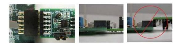
Figure 2. Pmod™ Connector Alignment
