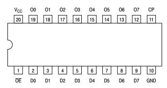
Figure 1. Pinout: 20-Lead (Top View)
