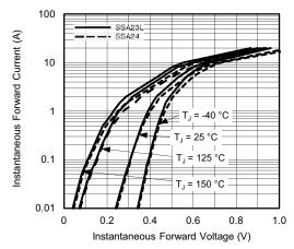
Fig. 3 - Typical Instantaneous Forward Characteristics
