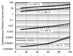
Fig. 4 - Typical Reverse Characteristics
