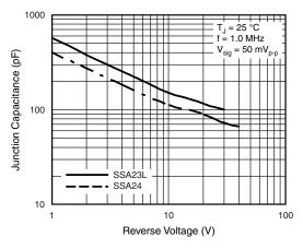
Fig. 5 - Typical Junction Capacitance
