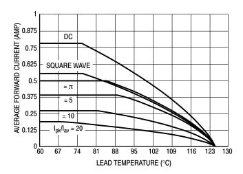
Figure 4. Current Derating (Lead)
