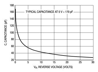
Figure 3. Typical Capacitance
