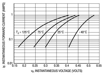
Figure 1. Typical Forward Voltage
