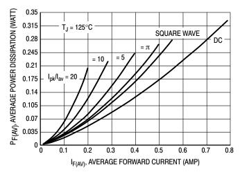
Figure 5. Power Dissipation
