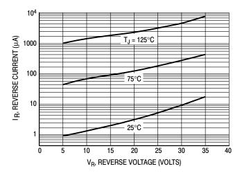
**Figure 2. Typical Reverse Current**
