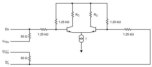
Figure 10. Input Structure
