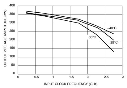
Figure 4. Output Voltage Amplitude ( $V_{OUTPP}$ ) versus Input Clock Frequency ( $f_{in}$ ) and Temperature (@  $V_{CC}$  = 3.3 V)
