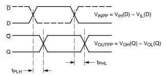
Figure 17. AC Reference Measurement
