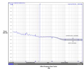
Figure 6. Typical Phase Noise Plot at f<sub>carrier</sub> = 622.08 MHz
