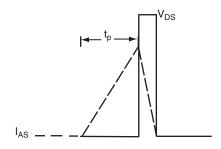
Fig. 12b - Unclamped Inductive Waveforms
