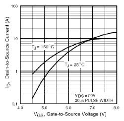
Fig. 3 - Typical Transfer Characteristics
