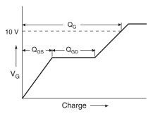
Fig. 12d - Basic Gate Charge Waveform
