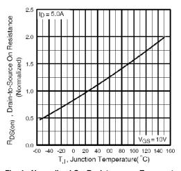
Fig. 4 - Normalized On-Resistance vs. Temperature
