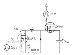
Fig. 12a - Unclamped Inductive Test Circuit
