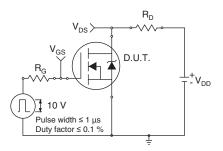
Fig. 10a - Switching Time Test Circuit
