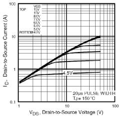
Fig. 2 - Typical Output Characteristics
