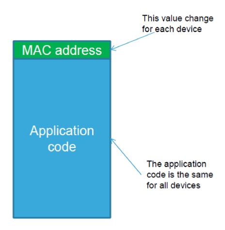
The BlueNRG-1, BlueNRG-2 devices do not have a valid preassigned MAC address, but a unique serial number (read only for the user). The unique serial number is a six byte value stored at address 0x100007F4: it is stored as two words (8 bytes) at address 0x100007F4 and 0x100007F8 with unique serial number padded with 0xAA55.
