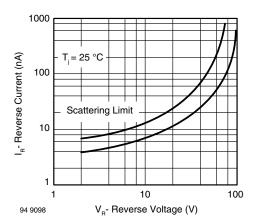
Fig. 3 - Reverse Current vs. Reverse Voltage
