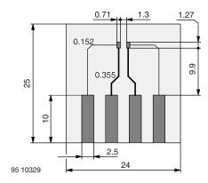
Fig. 5 - Board for RthJA definition (in mm)
