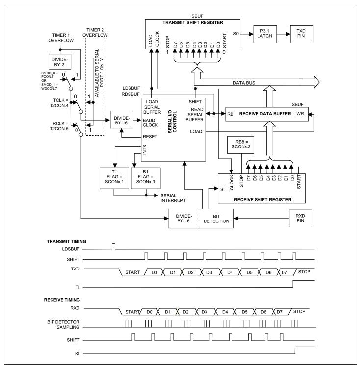
Figure 12-2. Serial Port Mode 1
