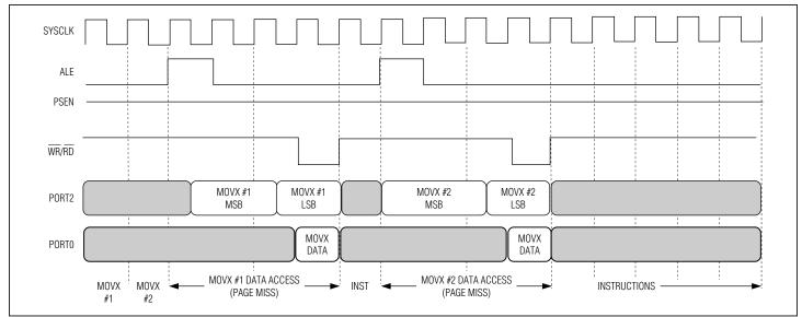
Figure 6-15. Two-Cycle Page Mode 1: MOVX (Two Cycles)
