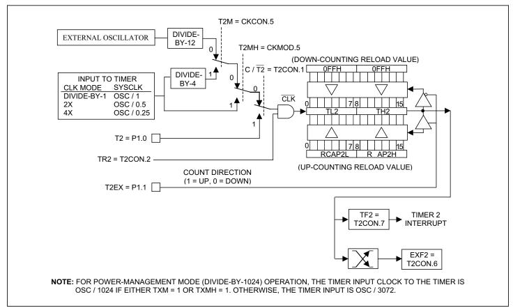
Figure 11-6. Timer/Counter 2 Autoreload Mode (DCEN = 1)
