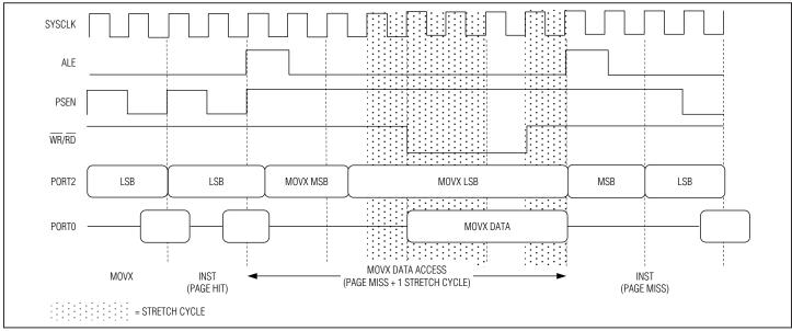
Figure 6-17. Two-Cycle Page Mode 1: MOVX (Three Cycles) External Code Execution with Page Misses
