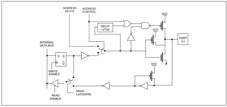
Figure 10-2. Port 2 Functional Circuitry
