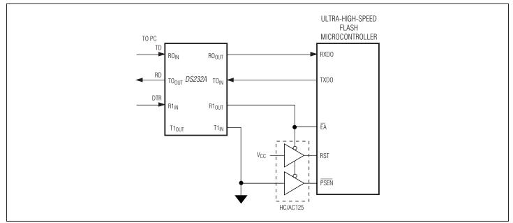
Figure 15-2. Serial Load Hardware Configuration
