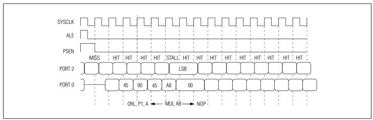
Figure 5-18. One-Cycle Page Mode 1: (Page Miss) - ORL Direct, A (Two Cycles) - ORL, A (Three Cycles) - NOP
