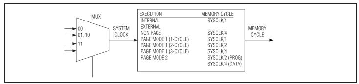
Figure 5-4. Instruction Memory Cycle Determination
