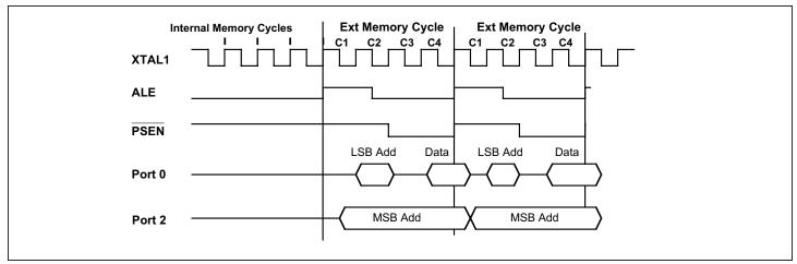
Figure 10-3. External Program Memory Access (Nonpage Model)
