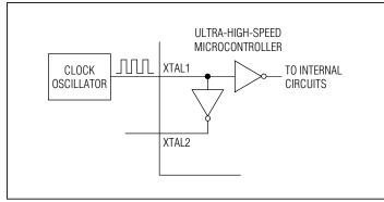
Figure 5-2. Clock Source Input
