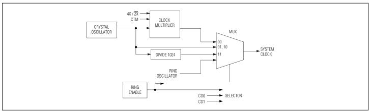
Figure 5-3. System Clock Sources
