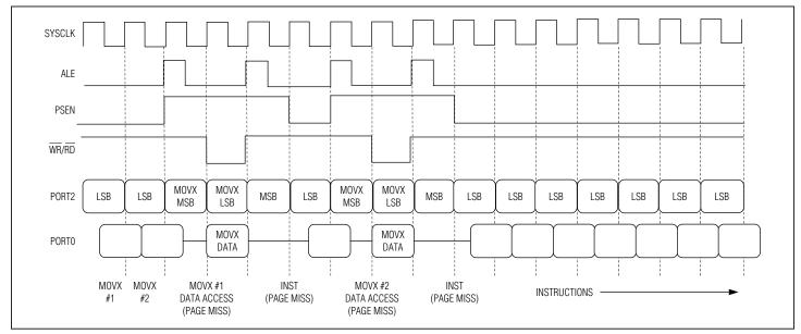
Figure 6-21. One-Cycle Page Mode 1: MOVX (Two Cycles)—MOVX (Two Cycles) External Code Execution
