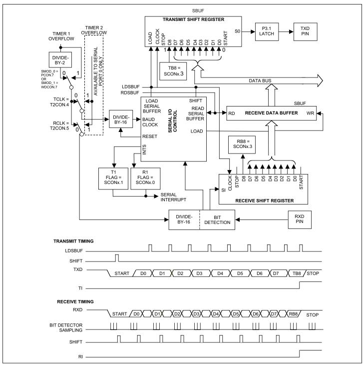
Figure 12-4. Serial Port Mode 3
