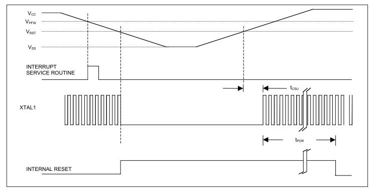
Figure 7-1. Power Cycle Operaton
