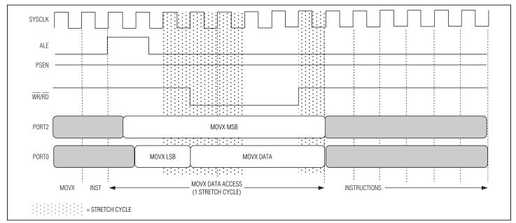
Figure 6-12. Nonpage Mode: MOVX (Three Cycles)
