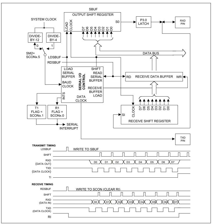
Figure 12-1. Serial Port Mode 0
