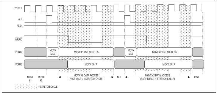
Figure 6-19. One-Cycle Page Mode 1: MOVX (Three Cycles)—MOVX (Three Cycles)
