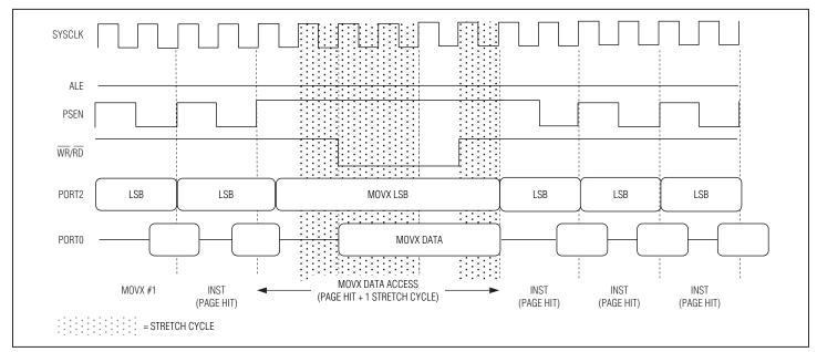
Figure 6-18. Two-Cycle Page Mode 1: MOVX (Three Cycles) External Code Execution - No Page Misses
