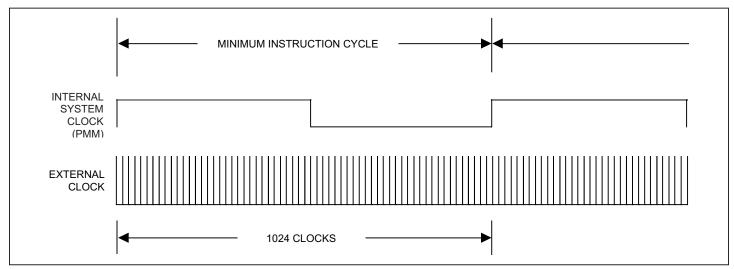
Figure 7-3. Internal Timing Relationships in PMM
