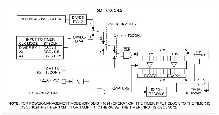
Figure 11-4. Timer/Counter 2 with Optional Capture (CP/RL2 = 1)
