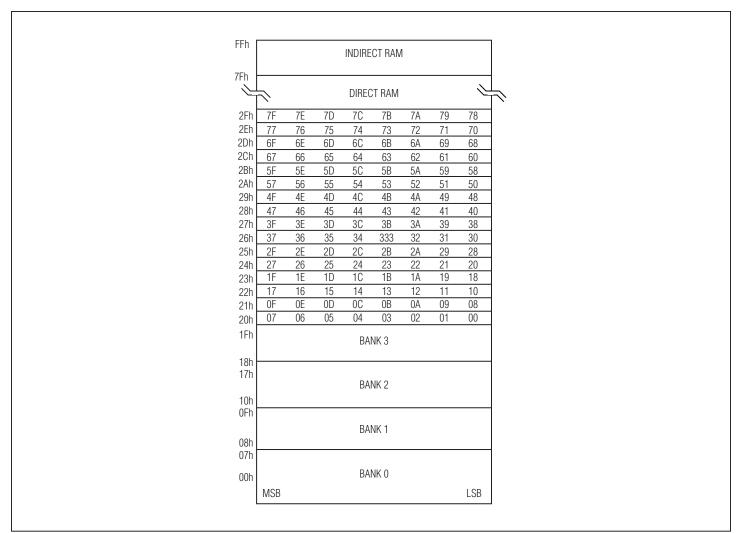
Figure 4-3. Scratchpad Register Addressing
