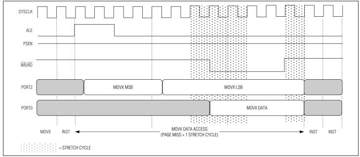
Figure 6-14. Four-Cycle Page Mode 1: MOVX (Three Cycles)
