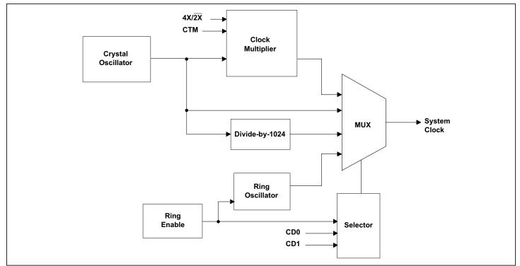
Figure 7-2. System Clock Sources
