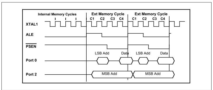
Figure 6-3. External Program Memory Access (Nonpage Mode and CD1:0 = 10b)
