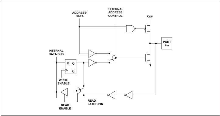
Figure 10-1. Port 0 Functional Circuitry
