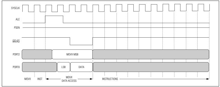
Figure 6-11. Nonpage Mode: MOVX (Two Cycles)
