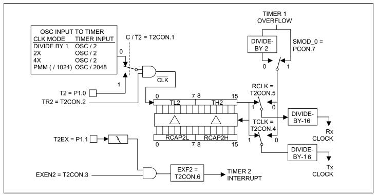
Figure 11-7. Timer/Counter 2 Baud-Rate Generator Mode
