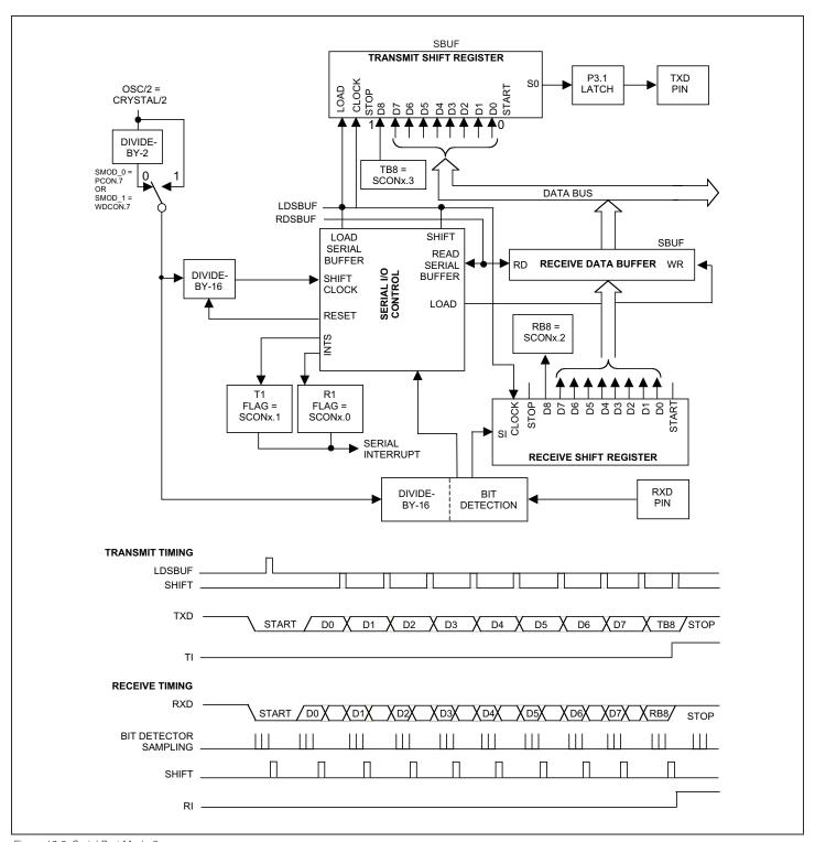
Figure 12-3. Serial Port Mode 2
