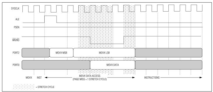
Figure 6-16. Two-Cycle Page Mode 1: MOVX (Three Cycles)
