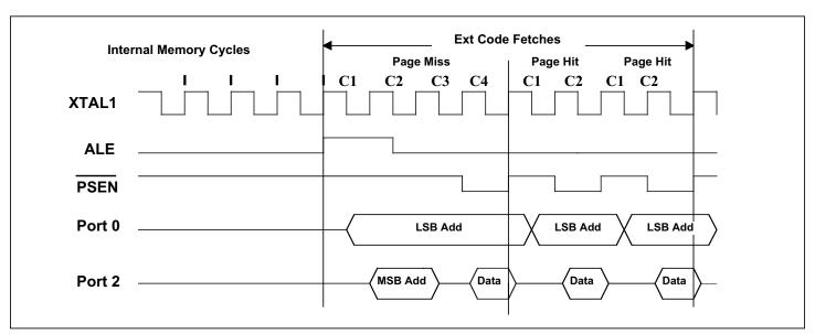
Figure 6-7. Page Mode 2 External Code Fetch Cycle (CD1:0 = 10b)
