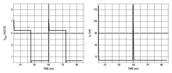
Figure 18. 20 Hz Square Wave Response
