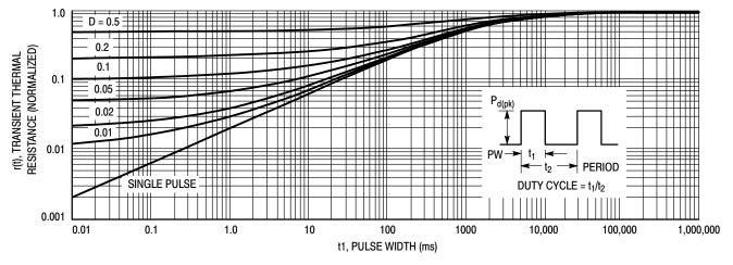
Figure 12. Transient Thermal Response for MDC3105LT1
