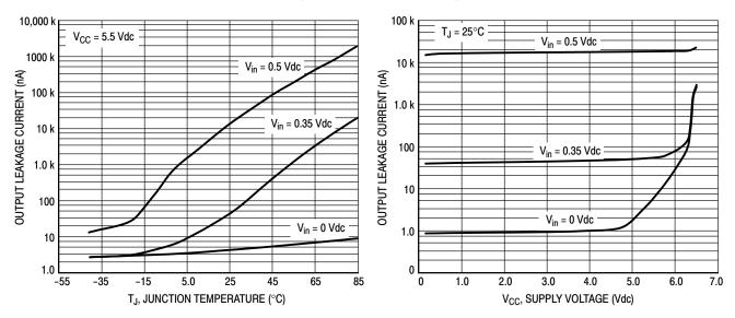
Figure 8. Output Leakage Current versus Temperature
