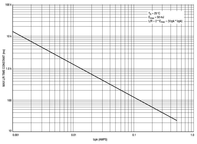
Figure 11. Zener Repetitive Pulse Energy Limit on L/R Time Constant for MDC3105LT1
