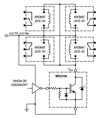
Figure 15. A Quad 5.0 V, 360 mW Coil Relay Bank
