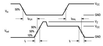
Figure 1. Switching Waveforms
