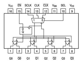
Figure 1. Logic Diagram and Pinout Assignment
