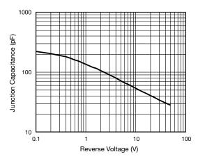
Fig. 5 - Typical Junction Capacitance
