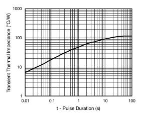
Fig. 6 - Typical Transient Thermal Impedance
