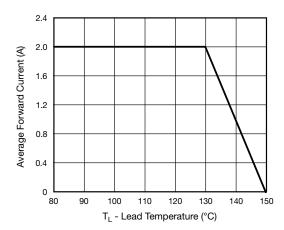
Fig. 1 - Forward Current Derating Curve
