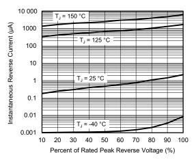
Fig. 4 - Typical Reverse Leakage Characteristics
