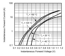
Fig. 3 - Typical Instantaneous Forward Characteristics
