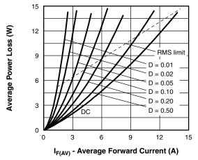
Fig. 6 - Forward Power Loss Characteristics
