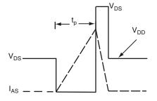
Fig. 12b - Unclamped Inductive Waveforms
