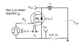
Fig. 12a - Unclamped Inductive Test Circuit
