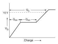
Fig. 13a - Basic Gate Charge Waveform
