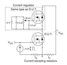
Fig. 13b - Gate Charge Test Circuit
