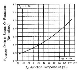
Fig. 4 - Normalized On-Resistance vs. Temperature
