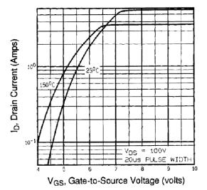
Fig. 3 - Typical Transfer Characteristics
