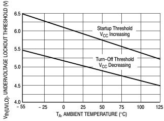
Figure 12. Undervoltage Lockout Threshold versus Temperature
