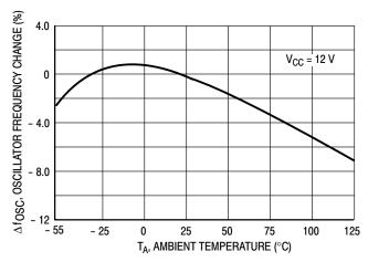
Figure 6. Oscillator Frequency Change versus Temperature
