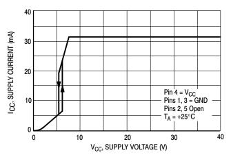
Figure 13. Operating Supply Current versus Supply Voltage
