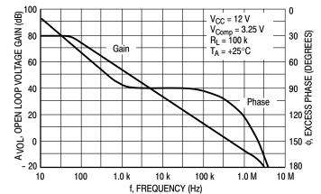
Figure 4. Error Amp Open Loop Gain and Phase versus Frequency
