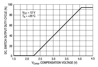
Figure 7. Switch Output Duty Cycle versus Compensation Voltage
