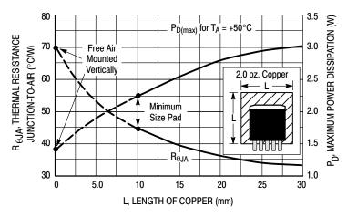
Figure 29. D<sup>2</sup>PAK Thermal Resistance and Maximum Power Dissipation versus P.C.B. Copper Length
