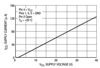
Figure 11. Standby Supply Current versus Supply Voltage
