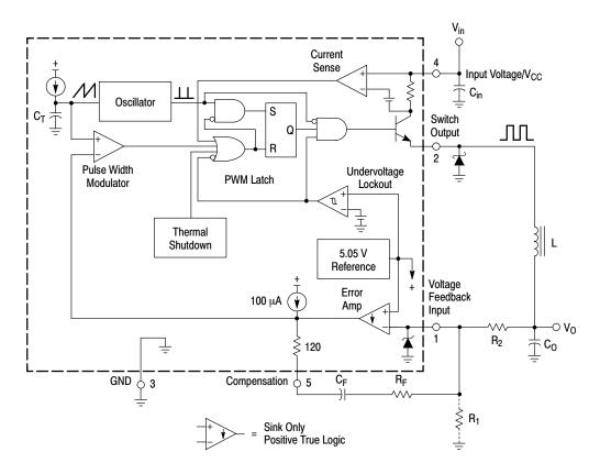
Figure 14. MC34166 Representative Block Diagram
