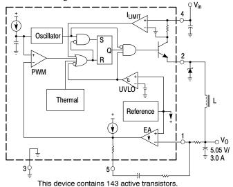
Figure 1. Simplified Block Diagram (Step Down Application)
