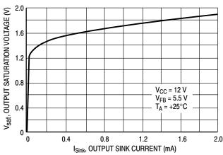
Figure 5. Error Amp Output Saturation versus Sink Current
