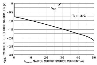
Figure 8. Switch Output Source Saturation versus Source Current
