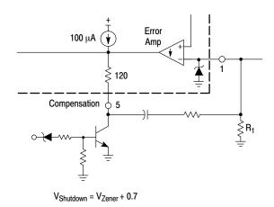
Figure 17. Over Voltage Shutdown Circuit
