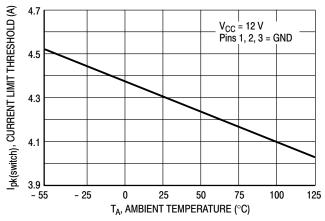
Figure 10. Switch Output Current Limit Threshold versus Temperature
