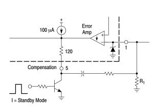
Figure 16. Low Power Standby Circuit
