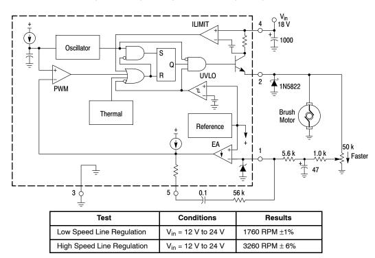
Figure 27. Variable Motor Speed Control with EMF Feedback Sensing
