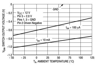
Figure 9. Negative Switch Output Voltage versus Temperature
