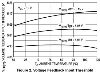
Figure 2. Voltage Feedback Input Threshold versus Temperature
