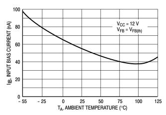
Figure 3. Voltage Feedback Input Bias Current versus Temperature
