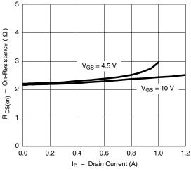
On-Resistance vs. Drain Current
