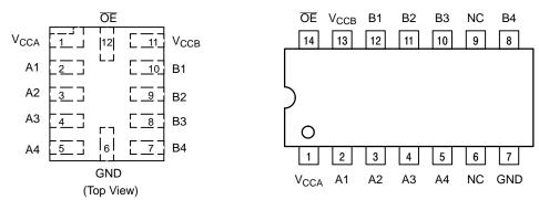
Figure 1. Pin Assignments
