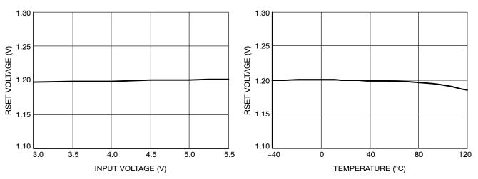
Figure 9. RSET Pin Voltage vs. Input Voltage
