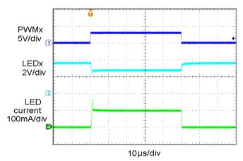
Figure 13. PWMx Transient Response
