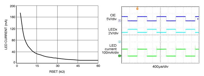
Figure 11. LED Current vs. RSET Resistor
