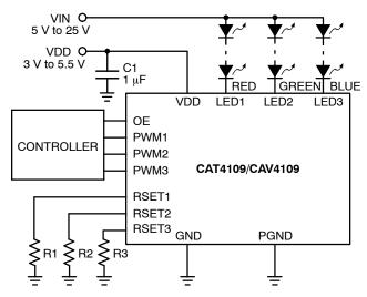
Figure 1. Typical Application Circuit
