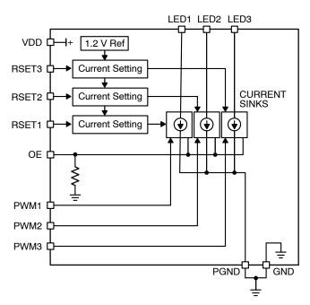
Figure 14. CAT4109/CAV4109 Functional Block Diagram
