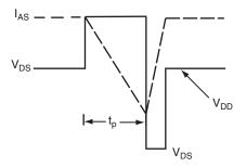
Fig. 12b - Unclamped Inductive Waveforms
