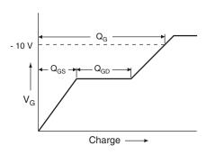
Fig. 13a - Basic Gate Charge Waveform
