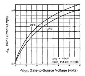
Fig. 3 - Typical Transfer Characteristics
