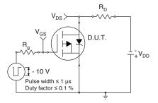
Fig. 10a - Switching Time Test Circuit
