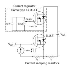
Fig. 13b - Gate Charge Test Circuit
