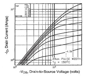
Fig. 2 - Typical Output Characteristics
