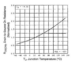
Fig. 4 - Normalized On-Resistance vs. Temperature
