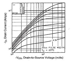
Fig. 1 - Typical Output Characteristics
