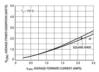
Figure 7. Power Dissipation
