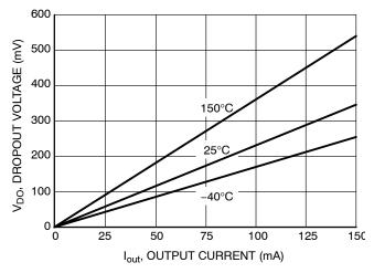
Figure 9. Dropout Voltage vs Output Current (5 V option)
