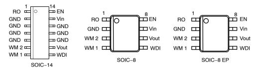
Figure 3. Pin Connections (Top View)
