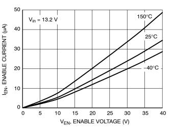
Figure 21. Enable Current vs. Enable Voltage
