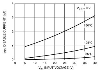
Figure 20. Disable Current vs. Input Voltage
