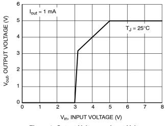
Figure 8. Output Voltage vs Input Voltage (5 V option)
