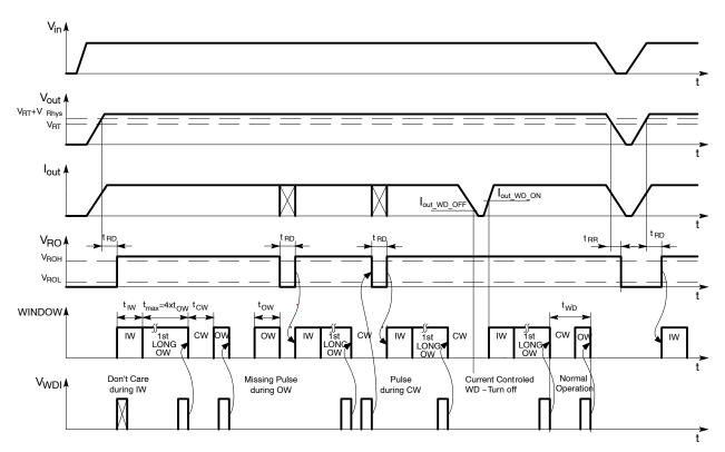
Figure 26. Window Watchdog Signal Diagram
