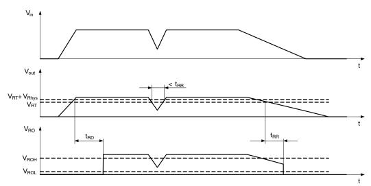
Figure 24. Reset Function and Timing Diagram
