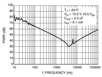
Figure 17. PSRR vs. Frequency (5 V option)
