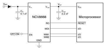
Figure 1. Application Schematic
