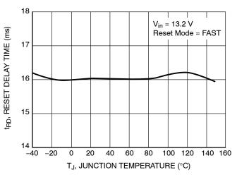
Figure 23. Reset Delay Time vs Temperature
