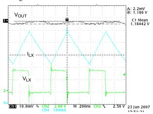
Figure 13. PWM Switching Waveforms ( $V_{IN} = 3.6 \text{ V}$ ,  $V_{OUT} = 1.2 \text{ V}$ ,  $I_{OUT} = 600 \text{ mA}$ , Temp = 25°C)
