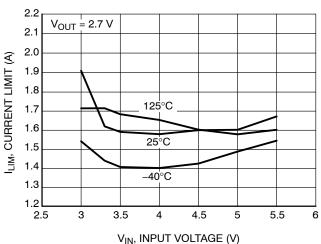
Figure 12. Peak Current Limit vs. Input Voltage
