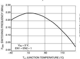
Figure 11. Switching Frequency vs.
