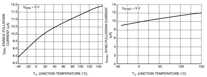
Figure 9. Enable Pulldown Current vs. Temperature
