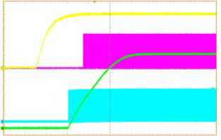
$\begin{array}{l} \mbox{CH1} = \mbox{EN} \ (0.5 \mbox{V/div}), \ \mbox{CH2} = \mbox{SW} \ (20 \mbox{V/div}), \ \mbox{CH3} = \mbox{LG} \ (2 \mbox{V/div}), \\ \mbox{CH4} = \mbox{Vo} \ (5 \mbox{V/div}), \ \mbox{T} = \mbox{2mS/Div} \end{array}$
