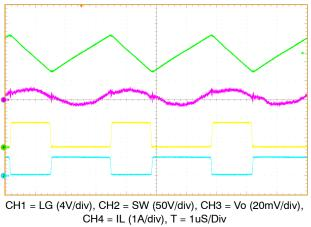
Figure 32. Switching and Voltage Ripple
