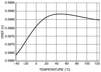
Figure 9. V<sub>REF</sub> vs T at V<sub>HVBIAS</sub> = 48 V
