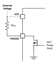
Figure 44. PGOOD Block Diagram
