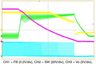
CH1 = FB (0.2V/div), CH2 = SW (20V/div), CH3 = Vo (5V/div), CH4 = IL (2A/div), T = 100uS/Div Figure 31. UVP due to Deep Over-current
