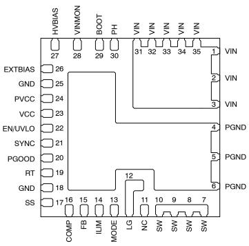
Figure 3. Pin Assignment (Bottom View)
