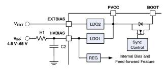
Figure 39. LDO Block Diagram
