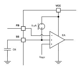
Figure 41. Soft Start Block Diagram
