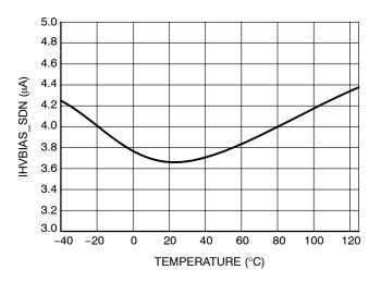
Figure 6. Shutdown Current vs. T at V<sub>HVBIA</sub>S = 48 V
