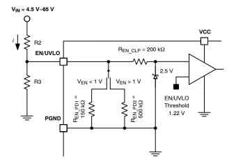
Figure 40. EN/UVLO Block Diagram
