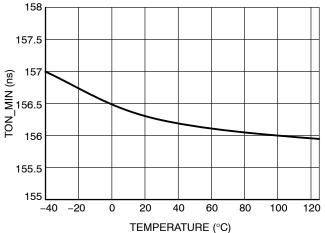
Figure 17. T<sub>ON MIN</sub> vs. T at  $V_{HVBIAS}$  = 48 V
