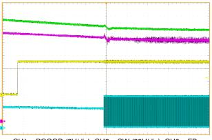
Figure 30. OVP1 Release at V<sub>FB</sub> ≤ 110% V<sub>REF</sub>
