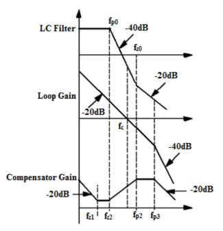
Figure 45. Power Stage, Loop Gain and Compensator Bode Plots
