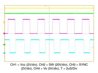
Figure 25. SYNC Output Frequency Duty Cycle in Master Mode
