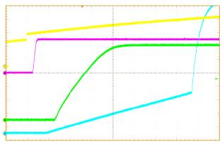
CH1 = EN (0.5V/div), CH2 = SS (0.5V/div), CH3 = Vcc (2V/div), CH4 = Vo (5V/div), T = 2mS/Div
