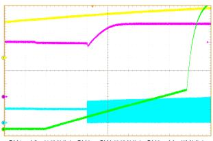
CH1 = Vin (10V/div), CH2 = SW (20V/div), CH3 = Vo (5V/div), CH4 = SS (0.5V/div), T = 2mS/Div Figure 23. System Startup with 75% Pre-bias
