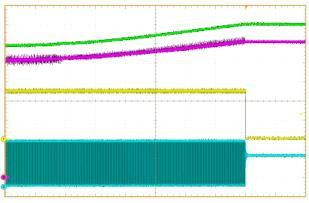
CH1 = PGOOD (2V/div), CH2 = SW (20V/div), CH3 = FB (0.1V/div), CH4 = Vo (4V/div), T = 500uS/Div
