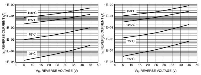
Figure 3. Typical Reverse Current
