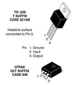
Heatsink surface (shown as terminal 4 in case outline drawing) is connected to Pin 2.
