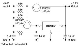
Figure 9. Current Boost Regulator (-5.0 V @ 4.0 A, with 5.0 A Current Limiting)
