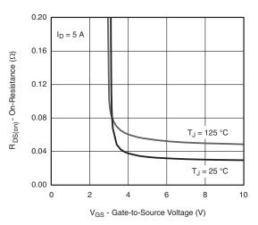
On-Resistance vs. Gate-to-Source Temperature
