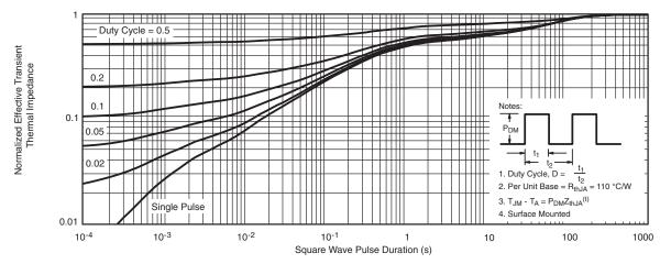
Normalized Thermal Transient Impedance, Junction-to-Ambient
