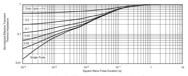
Normalized Thermal Transient Impedance, Junction-to-Foot
