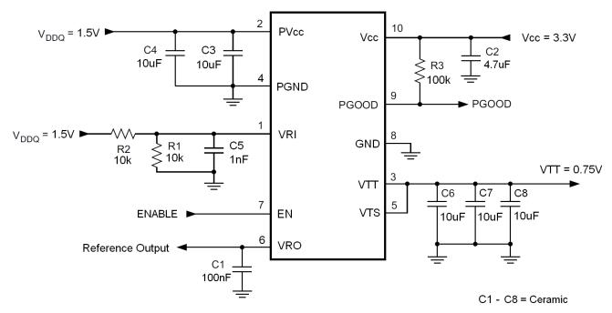
Figure 1. Typical DDR-3 Application Schematic
