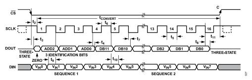
Figure 27. Writing to Shadow Register Timing Diagram
