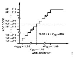
Figure 18. Twos Complement Transfer Characteristic with REF<sub>IN</sub> ± REF<sub>IN</sub> Input Range
