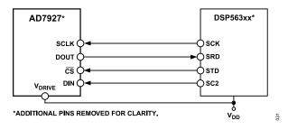
Figure 31. Interfacing to the DSP563xx
