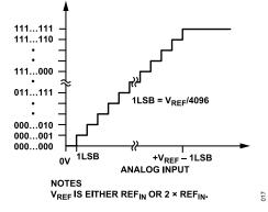
Figure 17. Straight Binary Transfer Characteristic
