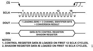
Figure 21. Normal Mode Operation
