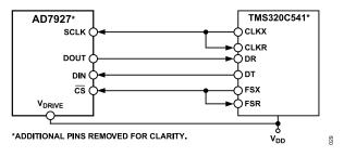
Figure 29. Interfacing to the TMS320C541
