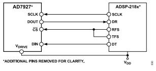
Figure 30. Interfacing to the ADSP-218x
