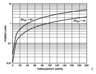
Figure 25. Power vs. Throughput Rate
