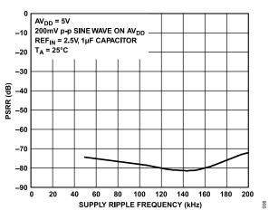
Figure 6. PSRR vs. Supply Ripple Frequency
