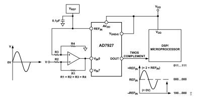
Figure 19. Handling Bipolar Signals
