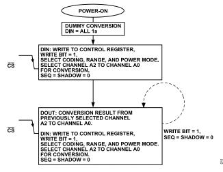
Figure 11. SEQ Bit = 0, SHADOW Bit = 0 Flowchart
