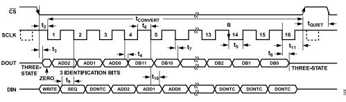
Figure 26. Serial Interface Timing Diagram
