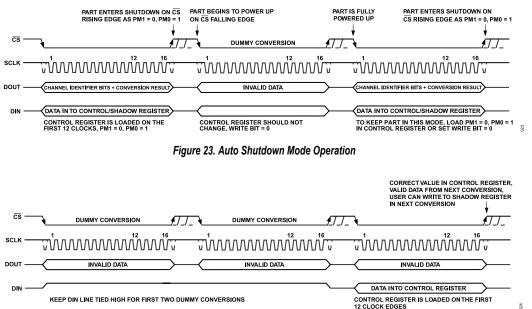
Figure 24. Three-Dummy-Conversions to Place AD7927 into the Required Operating Mode After Power Supplies Are Applied
