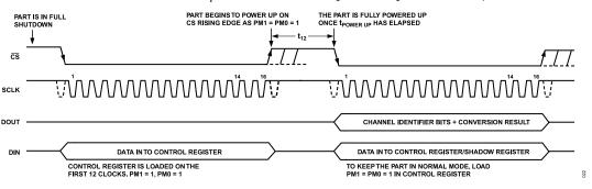
Figure 22. Full Shutdown Mode Operation
