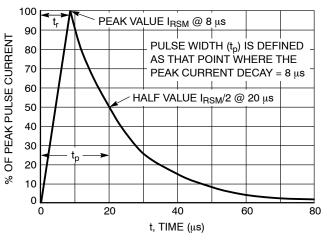
Figure 2. 8 X 20 µs Pulse Waveform
