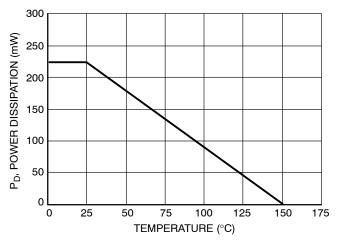
Figure 1. Steady State Power Derating Curve
