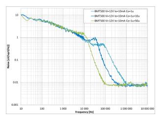
Figure 16. Noise – FIX – 5.0 V,  $I_{OUT}$  = 10 mA, Different  $C_{OUT}$
