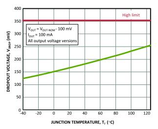
Figure 12. Dropout Voltage vs. Temperature
