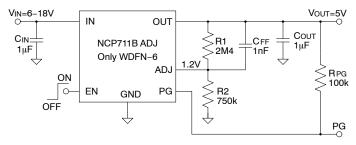
Figure 3. Fixed Output Voltage Application with PG
