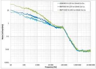
Figure 18. Noise – FIX,  $I_{OUT}$  = 10 mA,  $C_{OUT}$  = 1  $\mu F$ , Different  $V_{OUT}$
