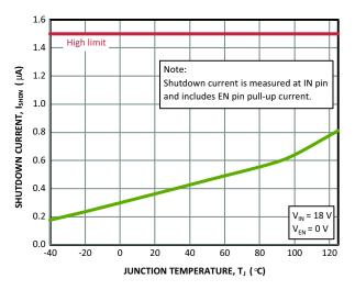
Figure 8. Shutdown Current vs. Temperature
