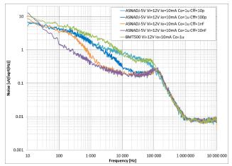
Figure 17. Noise – ADJ-set-5.0 V with Different C<sub>FF</sub> and FIX – 5.0 V
