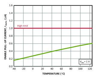
Figure 10. Enable Internal Pull-Up Current vs.
