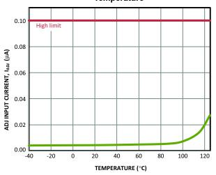
Figure 11. ADJ Input Current vs. Temperature
