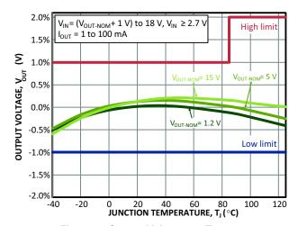
Figure 6. Output Voltage vs. Temperature
