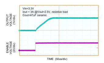
Figure 20. Enable Transient Response
