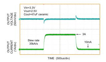
Figure 18. Load Transient Response
