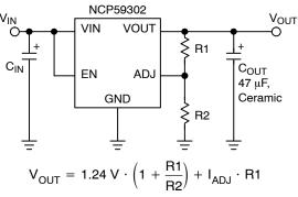
Figure 21. Adjustable Voltage Operation
