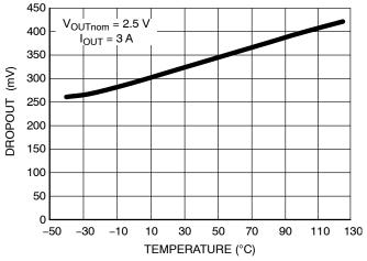
Figure 5. Dropout Voltage vs. Temperature
