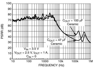
Figure 3. Power Supply Rejection Ratio
