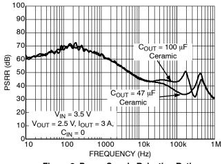
Figure 2. Power Supply Rejection Ratio
