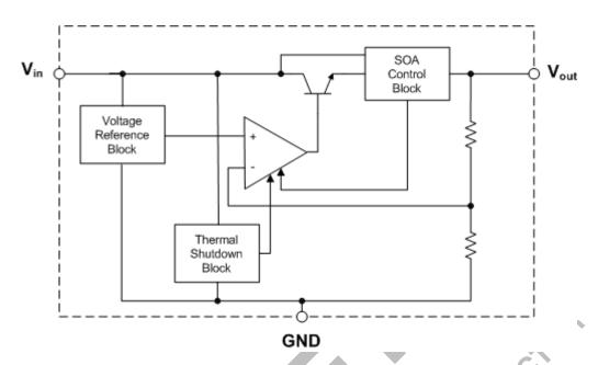
Figure 2. Simplified Block Diagram
