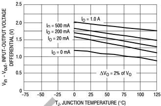
Figure 14. Input Output Differential as a Function of Junction Temperature
