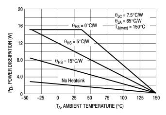
Figure 13. Worst Case Power Dissipation vs. Ambient Temperature (TO-220)
