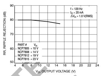
Figure 4. Ripple Rejection as a Function of Output Voltage
