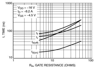
Figure 10. Resistive Switching Time Variation versus Gate Resistance
