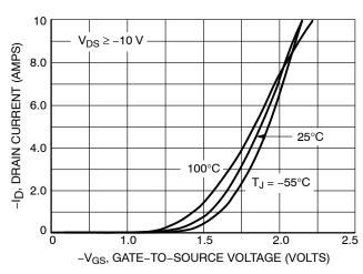
Figure 2. Transfer Characteristics
