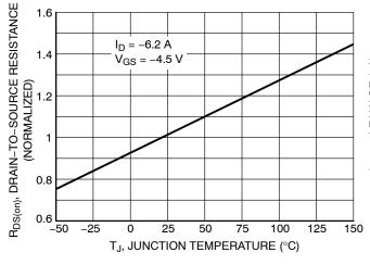
Figure 5. On–Resistance Variation with Temperature
