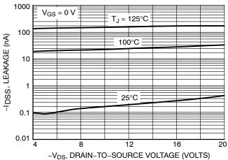
Figure 6. Drain-To-Source Leakage Current versus Voltage
