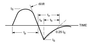
Figure 13. Diode Reverse Recovery Waveform
