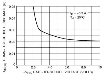
Figure 3. On-Resistance versus Gate-To-Source Voltage
