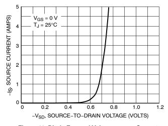
Figure 11. Diode Forward Voltage versus Current
