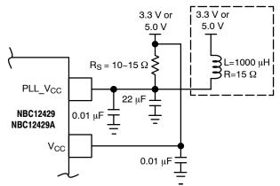
Figure 9. Power Supply Filter
