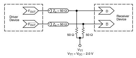
Figure 16. Typical Termination for Output Driver and Device Evaluation (See Application Note <u>AND8020/D</u> – Termination of ECL Logic Devices.)
