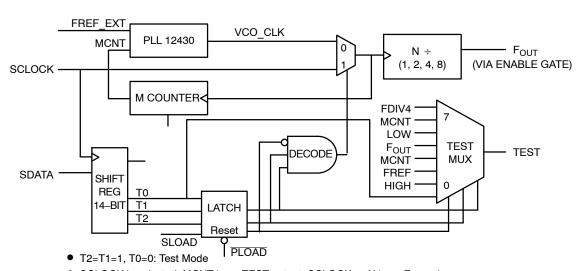
ullet SCLOCK is selected, MCNT is on TEST output, SCLOCK  $\div$  N is on F<sub>OUT</sub> pin. PLOAD acts as reset for test pin latch. When latch reset, T2 data is shifted out TEST pin.
