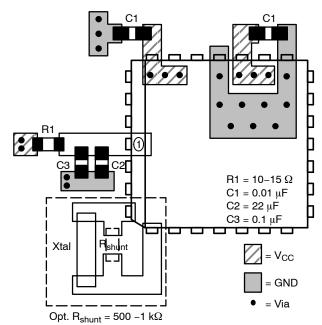
Figure 10. PCB Board Layout (PLCC-28)
