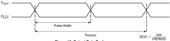
Figure 15. Output Duty Cycle
