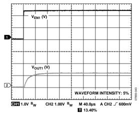
Figure 43. Typical Start-Up Time, Vout1 = 1.2 V
