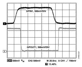
Figure 27. GPOUT1 Output vs. GPIN1 Input,  $V_{IN2}$  = 1.8 V,  $V_{IN3}$  = 1.2 V, 820  $\Omega$  Pull-Down, MSEL High, CH1 = GPIN1, CH2 = GPOUT1
