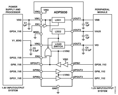
Figure 36. Application Diagram (MSEL Low)
