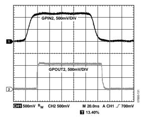
Figure 31. GPOUT2 Output vs. GPIN2 Input,  $V_{\rm IN2}$  = 1.8 V,  $V_{\rm IN3}$  = 1.2 V, 600  $\Omega$  Pull-Down, CH1 = GPIN2, CH2 = GPOUT2
