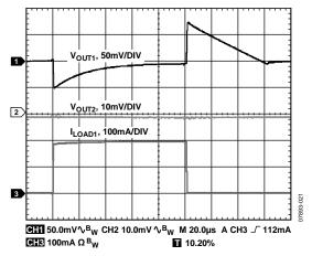
Figure 21. Load Transient Response,  $I_{LOAD1}=1$  mA to 200 mA,  $I_{LOAD2}=1$  mA,  $CH1=V_{OUT1}, CH2=V_{OUT2}, CH3=I_{LOAD1}, C_{OUT}=1$   $\mu F$
