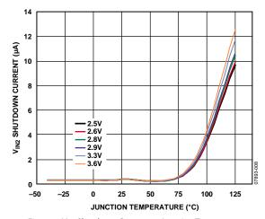
Figure 8. V<sub>IN2</sub> Shutdown Current vs. Junction Temperature at Various Input Voltages
