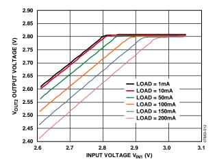
Figure 12. V<sub>OUT2</sub> Output Voltage vs. Input Voltage (in Dropout) and Load Current
