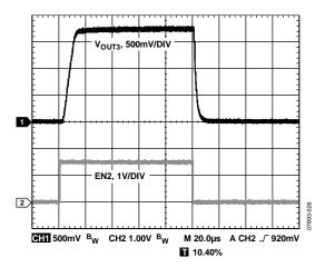
Figure 26. Load Switch Typical Switching Time,  $I_{LOAD3} = 100$  mA,  $CH1 = V_{OUT3}, CH2 = EN2$
