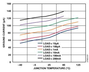
Figure 7. Ground Current vs. Junction Temperature, Both LDOs Loaded
