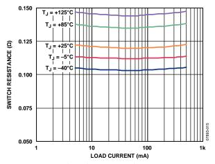
Figure 15. Load Switch RDS<sub>ON</sub> vs. Load Current,  $V_{IN2} = 1.8 \text{ V}$
