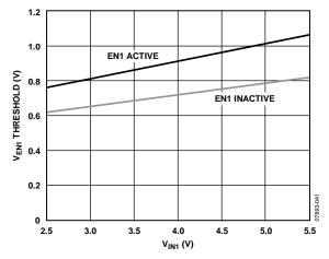
Figure 41. Typical EN1 Pin Thresholds vs. Input Voltage
