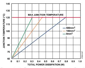
Figure 47. Junction Temperature vs. Total Power Dissipation,  $T_A = 65$  °C
