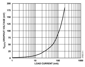
Figure 11. Vout2 Dropout Voltage vs. Load Current
