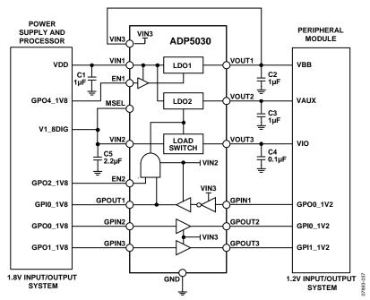
Figure 37. Application Diagram (MSEL High)
