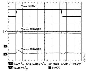
Figure 23. Line Transient Response,  $V_{IN1} = 4 \text{ V to 5 V}$ ,  $I_{LOAD1} = 1 \text{ mA}$ ,  $I_{LOAD2} = 1 \text{ mA}$ ,  $CH1 = V_{IN1}$ ,  $CH2 = V_{OUT1}$ ,  $CH3 = V_{OUT2}$
