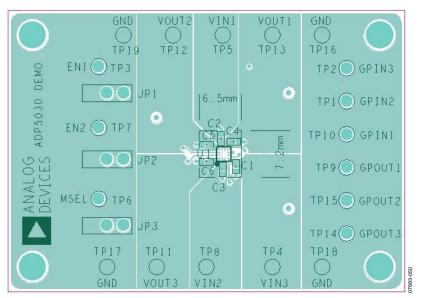
Figure 50. Example of PCB Layout, Top Side
