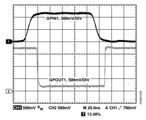
Figure 28. GPOUT1 Output vs. GPIN1 Input,  $V_{\rm IN2}$  = 1.8 V,  $V_{\rm IN3}$  = 1.2 V, 820  $\Omega$  Pull-Up, MSEL High, CH1 = GPIN1, CH2 = GPOUT1
