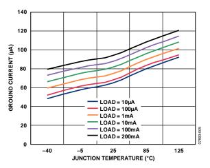
Figure 5. Ground Current vs. Junction Temperature, V<sub>OUT1</sub> Loaded
