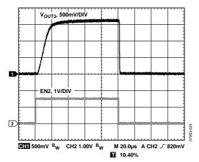
Figure 25. Load Switch Typical Switching Time,  $I_{LOAD3} = 500$  mA,  $CH1 = V_{OUT3}, CH2 = EN2$
