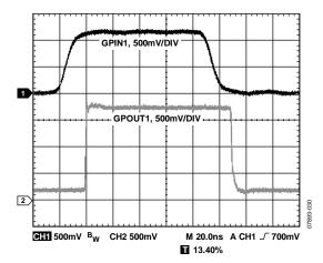
Figure 30. GPOUT1 Output vs. GPIN1 Input,  $V_{\rm IN2}$  = 1.8 V,  $V_{\rm IN3}$  = 1.2 V, 820  $\Omega$  Pull-Up, MSEL Low, CH1 = GPIN1, CH2 = GPOUT1
