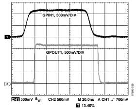
Figure 29. GPOUT1 Output vs. GPIN1 Input,  $V_{IN2}$  = 1.8 V,  $V_{IN3}$  = 1.2 V, 820  $\Omega$  Pull-Down, MSEL Low, CH1 = GPIN1, CH2 = GPOUT1
