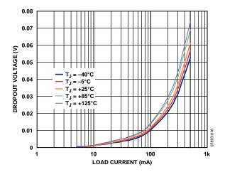
Figure 16. Load Switch Dropout Voltage vs. Load Current,  $V_{\text{IN2}} = 1.8 \text{ V}$
