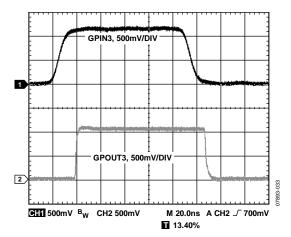
Figure 33. GPOUT3 Output vs. GPIN3 Input,  $V_{\rm IN2}$  = 1.8 V,  $V_{\rm IN3}$  = 1.2 V, 600  $\Omega$  Pull-Down, CH1 = GPIN3, CH2 = GPOUT3
