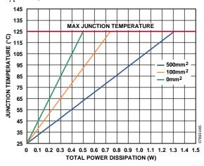
Figure 45. Junction Temperature vs. Total Power Dissipation,  $T_A = 25$ °C
