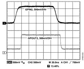
Figure 32. GPOUT2 Output vs. GPIN2 Input,  $V_{IN2}$  = 1.8 V,  $V_{IN3}$  = 1.2 V, 600  $\Omega$  Pull-Up, CH1 = GPIN2, CH2 = GPOUT2
