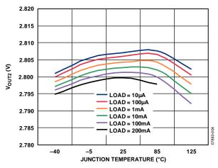
Figure 4. Vout2 Output Voltage vs. Junction Temperature
