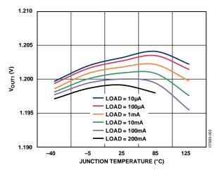
Figure 3. V<sub>OUT1</sub> Output Voltage vs. Junction Temperature
