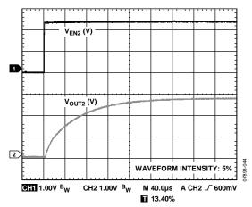
Figure 44. Typical Start-Up Time,  $V_{OUT2} = 2.8 \text{ V}$
