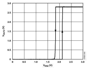
Figure 40. Typical EN2 Pin Operation
