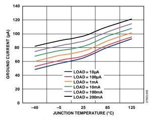
Figure 6. Ground Current vs. Junction Temperature, Vout2 Loaded
