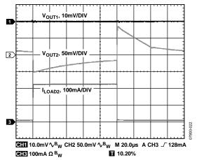
Figure 22. Load Transient Response,  $I_{LOAD1} = 1$  mA,  $I_{LOAD2} = 1$  mA to 200 mA,  $CH1 = V_{OUT1}$ ,  $CH2 = V_{OUT2}$ ,  $CH3 = I_{LOAD2}$
