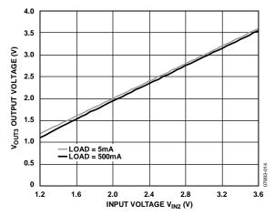
Figure 14. Load Switch (V<sub>OUT3</sub>) Output Voltage vs. Input Voltage and Load Current
