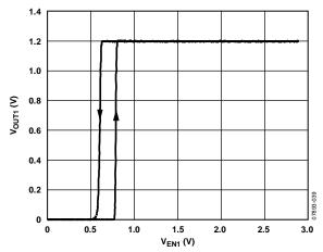
Figure 39. Typical EN1 Pin Operation
