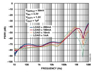
Figure 18. Power Supply Rejection Ratio vs. Frequency,  $V_{\text{INI}} = 3.3 \text{ V}$ ,  $V_{\text{OUTI}} = 1.2 \text{ V}$
