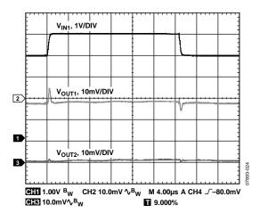
Figure 24. Line Transient Response,  $V_{INI} = 4 V$  to 5 V,  $I_{LOADI} = 200 mA$ ,  $I_{LOAD2} = 200 mA$ ,  $CH1 = V_{IN1}$ ,  $CH2 = V_{OUT1}$ ,  $CH3 = V_{OUT2}$
