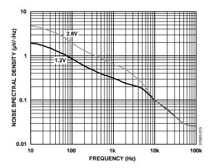
Figure 19. Output Noise Spectral Density vs. Output Voltage,  $V_{IN1} = 5 V$ ,  $I_{LOAD} = 10 \text{ mA}$
