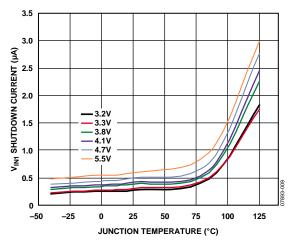
Figure 9. V<sub>IN1</sub> Shutdown Current vs. Junction Temperature at Various Input Voltages
