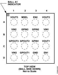
Figure 2. Pin Configuration, Top View
