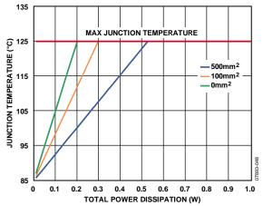
Figure 48. Junction Temperature vs. Total Power Dissipation,  $T_A = 85^{\circ}C$
