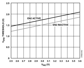
Figure 42. Typical EN2 Pin Thresholds vs. Input Voltage
