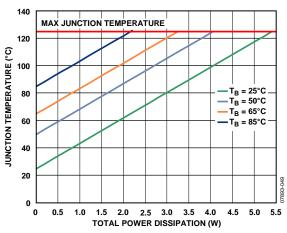
Figure 49. Junction Temperature vs. Total Power Dissipation and Board Temperature
