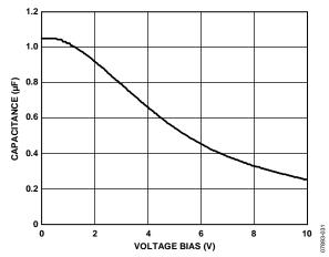
Figure 38. Capacitance vs. Voltage Bias Characteristics
