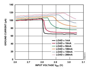
Figure 13. Ground Current for V<sub>OUT2</sub> (in Dropout) vs. Input Voltage and Load Current
