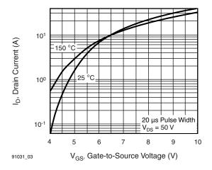
Fig. 3 - Typical Transfer Characteristics
