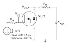
Fig. 10a - Switching Time Test Circuit
