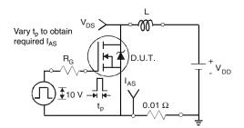
Fig. 12a - Unclamped Inductive Test Circuit
