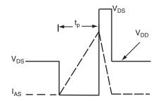
Fig. 12b - Unclamped Inductive Waveforms
