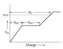
Fig. 13a - Basic Gate Charge Waveform
