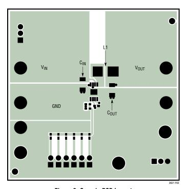
Figure 2. Sample PCB Layout
