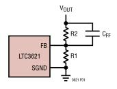
Figure 1. Setting the Output Voltage
