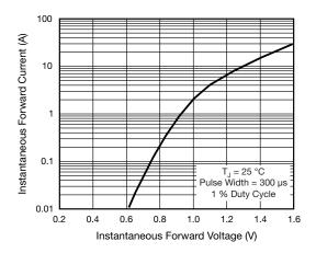
Fig. 3 - Typical Instantaneous Forward Characteristics
