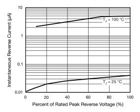
Fig. 4 - Typical Reverse Characteristics
