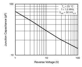
Fig. 5 - Typical Junction Capacitance
