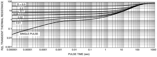
Figure 14. Thermal Response Junction-to-Ambient, per Leg for MBRF20L60CT
