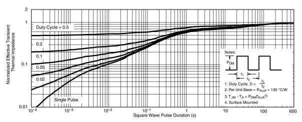
Normalized Thermal Transient Impedance, Junction-to-Ambient
