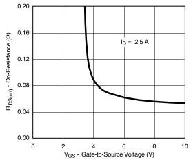
On-Resistance vs. Gate-to-Source Voltage
