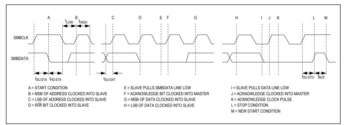
Figure 3. SMBus Write Timing Diagram
