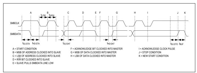
Figure 4. Read-Timing Diagram
