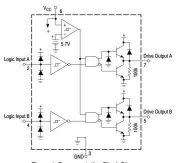
Figure 1. Representative Block Diagram
