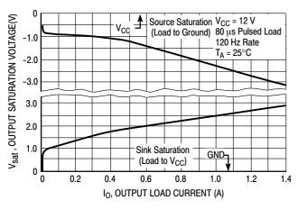
Figure 10. Drive Output Saturation Voltage versus Load Current
