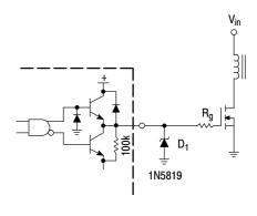
Series gate resistor  $\boldsymbol{R}_g$  may be needed to damp high frequency parasitic oscillations caused by the MOSFET input capacitance and any series wiring inductance in the gate–source circuit.  $\boldsymbol{R}_g$  will decrease the MOSFET switching speed. Schottky diode  $\boldsymbol{D}_1$  can reduce the driver's power dissipation due to excessive ringing, by preventing the output pin from being driven below ground.
