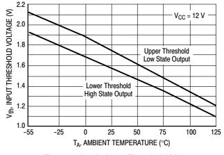
Figure 5. Logic Input Threshold Voltage versus Temperature
