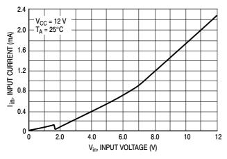
Figure 4. Logic Input Current versus Input Voltage
