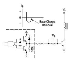
The totem-pole outputs can furnish negative base current for enhanced transistor turn-off, with the addition of capacitor  $C_1$ .
