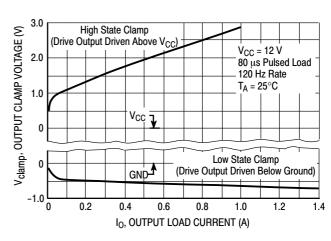
Figure 9. Drive Output Clamp Voltage versus Clamp Current
