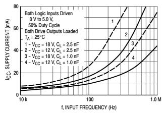
Figure 16. Supply Current versus Input Frequency
