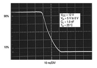
Figure 13. Drive Output Fall Time
