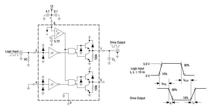
Figure 2. Switching Characteristics Test Circuit
