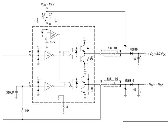
The capacitor's equivalent series resistance limits the Drive Output Current to 1.5 A. An additional series resistor may be required when using tantalum or other low ESR capacitors.
