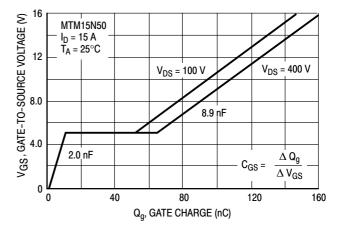
Figure 18. Gate-To-Source Voltage versus Gate Charge
