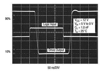
Figure 8. Propagation Delay
