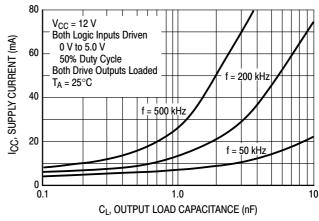
Figure 15. Supply Current versus Drive Output Load Capacitance
