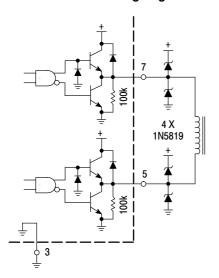
Output Schottky diodes are recommended when driving inductive loads at high frequencies. The diodes reduce the driver's power dissipation by preventing the output pins from being driven above V<sub>CC</sub> and below ground.
