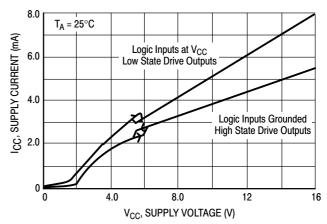
Figure 17. Supply Current versus Supply Voltage
