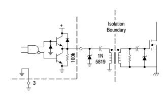
Figure 22. Isolated MOSFET Drive
