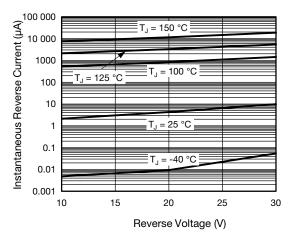
Fig. 4 - Typical Reverse Leakage Characteristics
