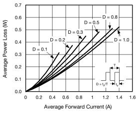
Fig. 2 - Forward Power Loss Characteristics
