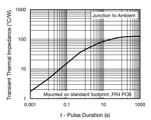
Fig. 6 - Typical Transient Thermal Impedance
