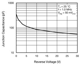
Fig. 5 - Typical Junction Capacitance
